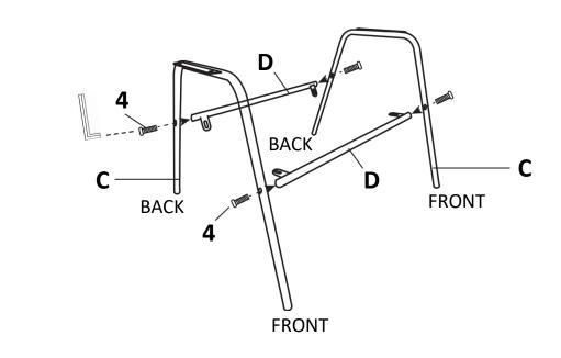
STEP 3: Turn over "CHAIR SEAT" assembled in "STEP 1" and place on top "METAL FRAME" assembled in "STEP 2". Align the eyelets on the metal frame with bolt holes on chair seat and assemble with M6\*30 bolts (4).
